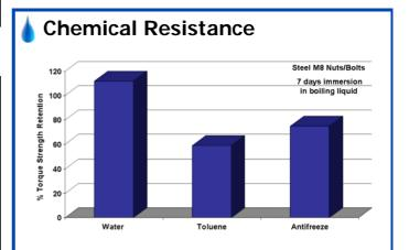
This product is not recommended for use in joints which will be in contact with either steam or pure oxygen. Avoid prolonged contact with strong acids, alkalis and very polar solvents
