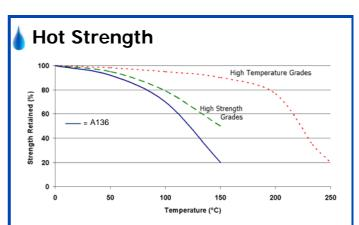
The reduction in strength shown here is reversed on cooling providing the joint is not overstressed. Exposure to higher temperatures may be acceptable for short periods
