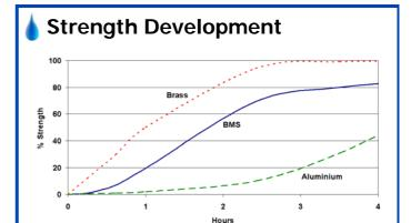
Cure times are typical at 23°C. Copper and its alloys will follow the faster cure while oxidised or passivated surfaces like stainless steel will tend towards the slower curve. Lower temperatures or large gaps will tend to extend the cure time. To reduce the cure time the use of Permabond A905, or heat, can be considered.
